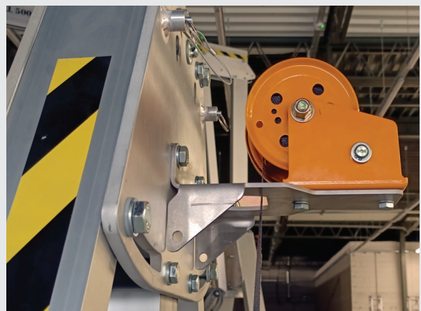
Simplifying the design of the hoist to the support (product ordered separately). Complete elimination of welded parts. Easier installation.
