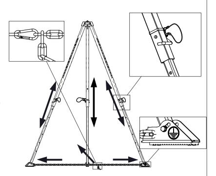
MAXIMUM LOAD TRANSMITTED FROM THE TM 7 TO THE STRUCTURE / LOADING DIRECTION
