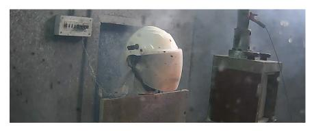
Shield after the test with traces of electric arc exposure.
