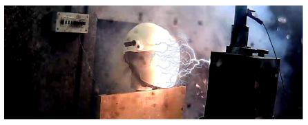
The effect of an electric arc on the surface of the shield (4 kA/0,5s) - class 1
