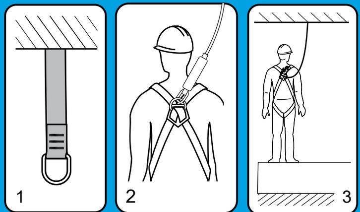
The webbing sling is designed to be installed in the middle of a reinforced concrete structure (reinforced concrete) in order to create a point for fastening safety harnesses. The webbing sling is intended for use by only one employee. The device has been tested and positively certified in accordance with EN 795: 2012 (Fall protection from height, Anchor devices, Requirements and tests, TYPE A).
